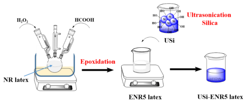
Figure 1. Diagram for preparation of ENR5 latex mixed with ultrasonicated silica particles
