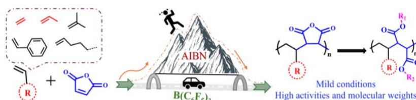
Figure 1. Control radical polymerization of olefins with maleic anhydride mediated by Lewis acid
