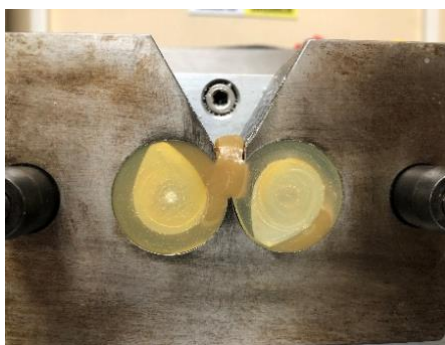
Fig. 1: The photograph of melt mixing device and a representative sample.
